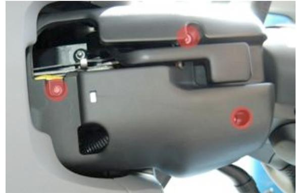
Lower the bottom steering wheel adjustment arm. You will need to move the steering column in and out as well as up and down to remove the lower piece of plastic.
