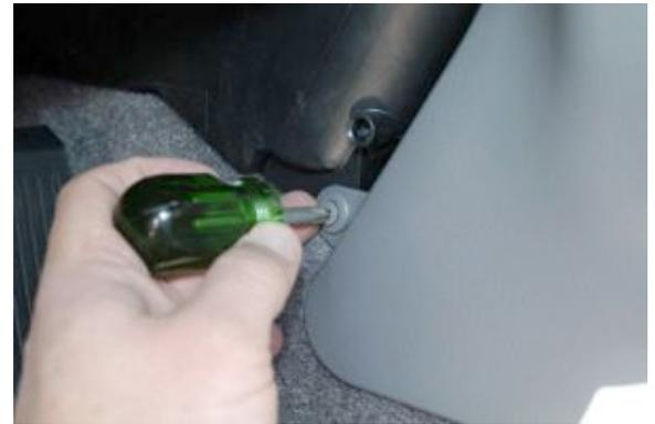
From the top section of the triangular panel, remove the metal Philips screw.
