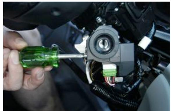
Make sure you have an unworn correctly sized Philips screwdriver as you do not want to burr the heads on these screws.
