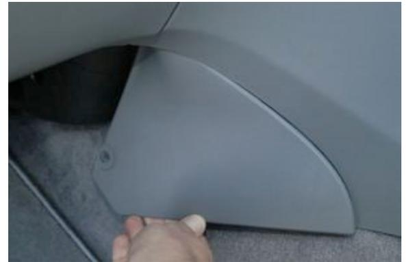
Pull back the carpet and undo the left 10mm bolt holding in the ECU.
