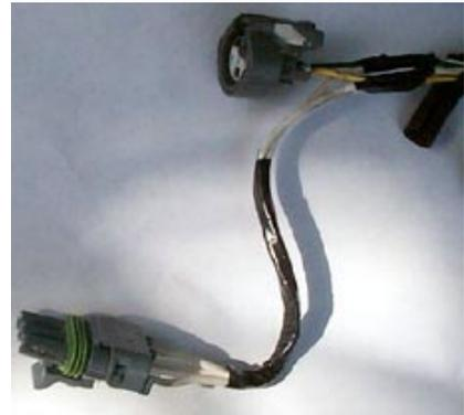
*3 Bar pigtail spliced into stock wiring*
