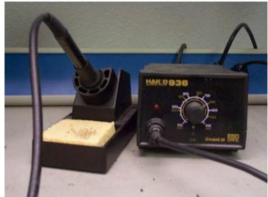
*Hakko 936 Temp controlled soldering iron*
